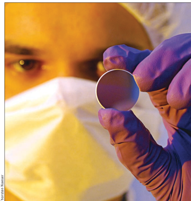
The laboratory for attosecond physics at Garching produces chirped multilayer mirrors for its research. Volodymyr Pervak (left) and Adrian Cavaliere (bottom middle) are seen examining the mirrors. An array of multilayer mirrors (top middle) compresses ultrabroadband laser pulses to 1.5 wave cycles. The attosecond X-ray pulses produced with them allow the control and real-time observation of atomic-scale electron motion. Lund's attosecond stroboscope is shown far right.
