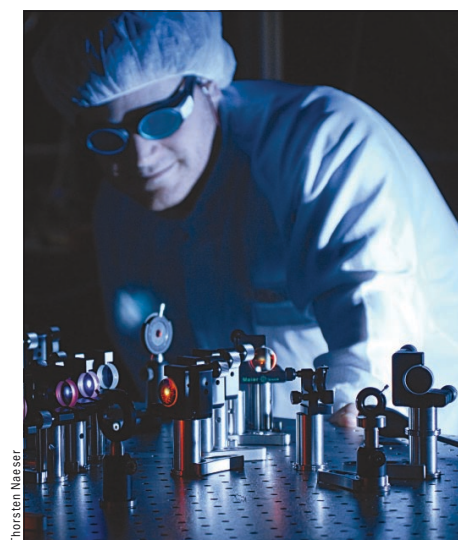
The laboratory for attosecond physics at Garching produces chirped multilayer mirrors for its research. Volodymyr Pervak (left) and Adrian Cavaliere (bottom middle) are seen examining the mirrors. An array of multilayer mirrors (top middle) compresses ultrabroadband laser pulses to 1.5 wave cycles. The attosecond X-ray pulses produced with them allow the control and real-time observation of atomic-scale electron motion. Lund's attosecond stroboscope is shown far right.
