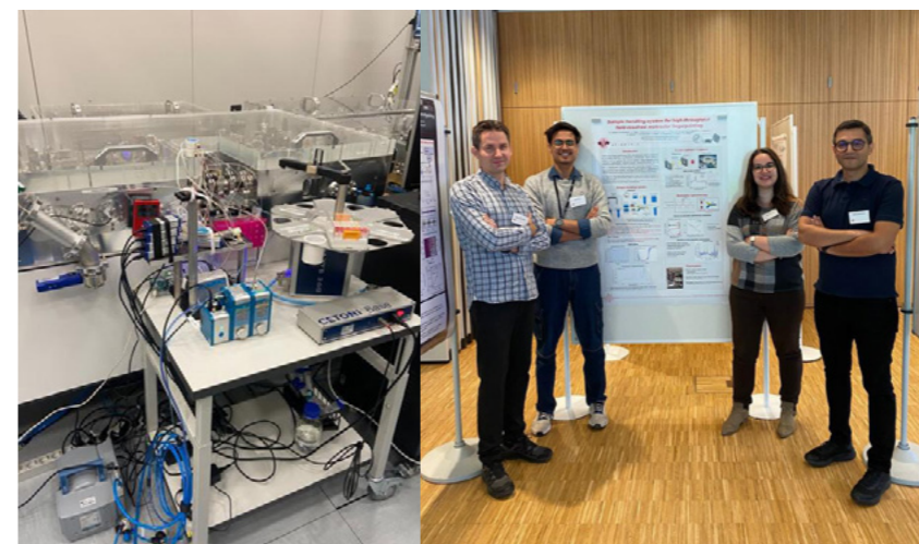
Left: Home-built automated sample handling system with modulated sample exchange. Right: Microfluidics team presenting at the ATTOWORLD-alumni meeting (from left to right: Dr. Igor Kukhtevich, Akash Singh, Dr. Elisa Lambert, Amaj Chamankar). Images: FRIS-team
