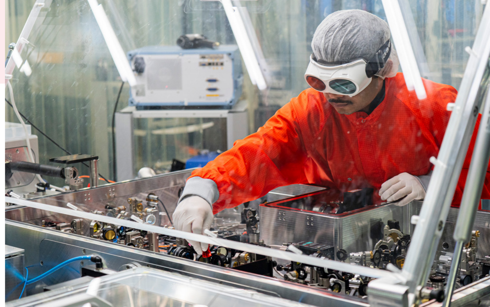
Abhijit Maity performs final checks on the recently upgraded Infrsampler 1.5 system before it is transported to the new CMF laboratory in Szeged. After reinstallation, it will be used to determine the electric-field molecular fingerprint of thousands of H4H samples. Photo: Thorsten Naeser
