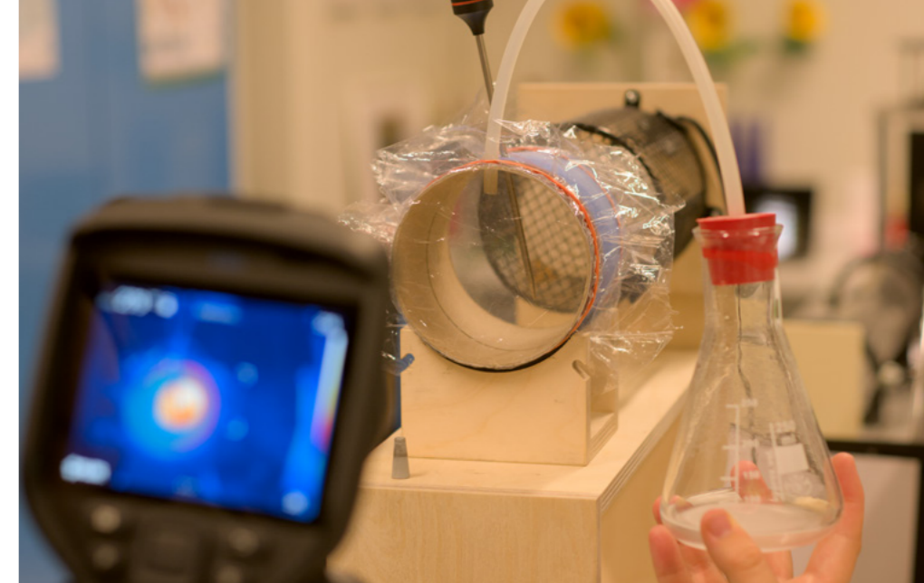
Filling the "infrared chamber" with CO 2 while watching this with the infrared camera. Photo: PhotonLab/Henry Hill
