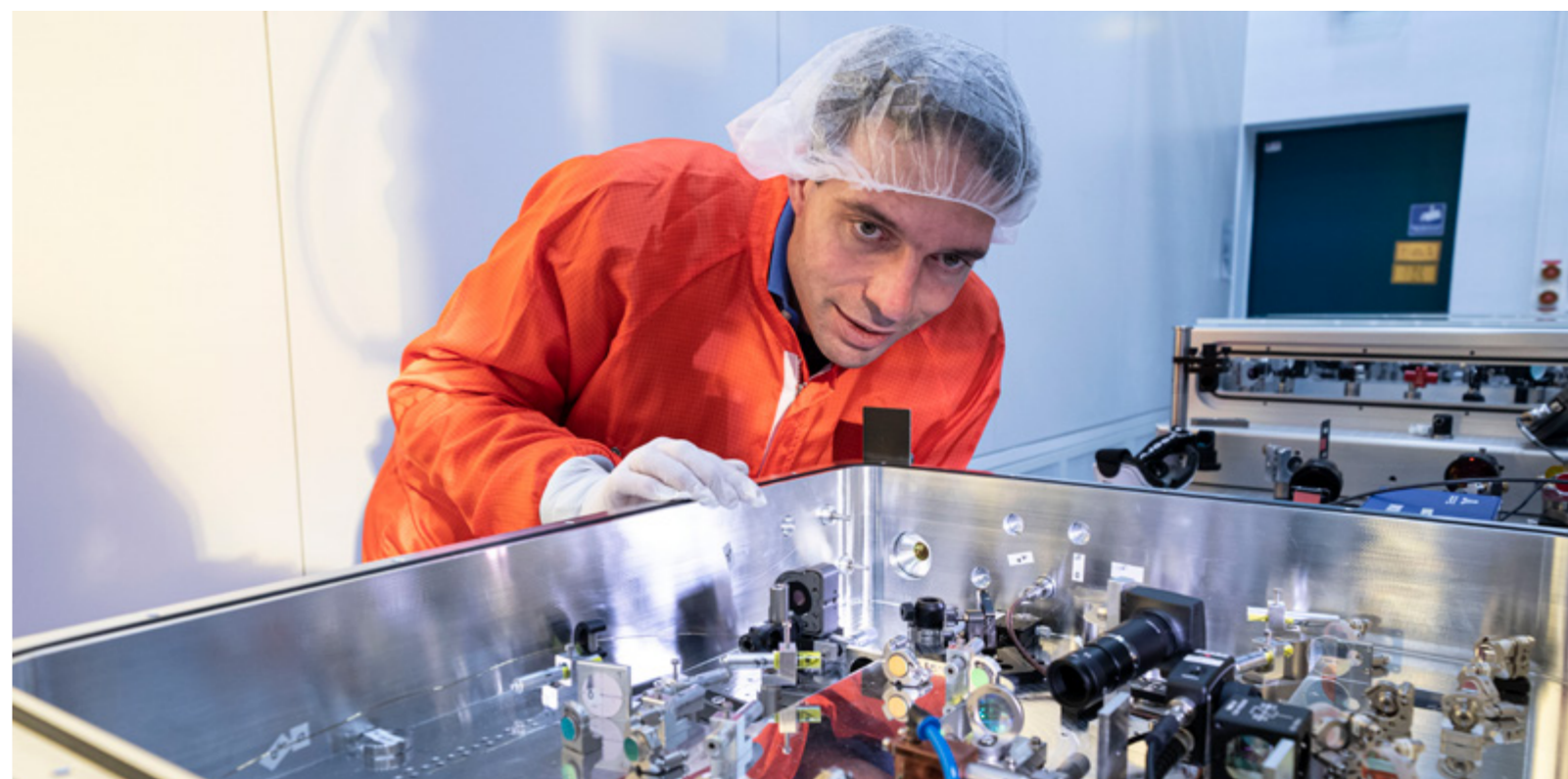
Inspecting the first prototype of the next-generation Cr:ZnS laser in the laboratory. Photos: Thorsten Naeser
